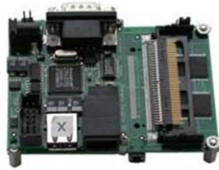
Figure 5: An Xscale(TM) architecture based gateway node
