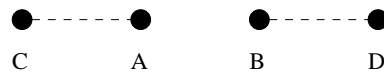
Fig. 2. Neighboring nodes A and B have different schedules. They synchronize with nodes C and D respectively.
