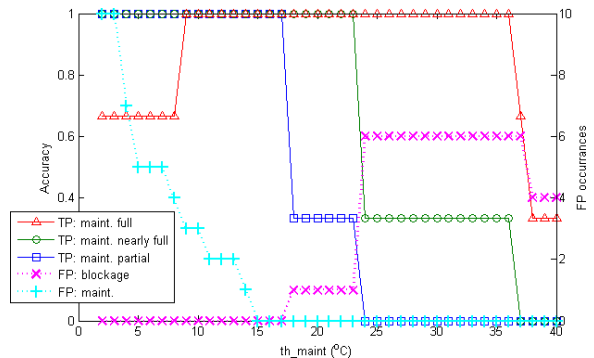
Figure 23: Evaluation of improved algorithm running between T_d^2 and T_d^3 for MAINTENANCE detection. th\_block is fixed at 15 °C.
